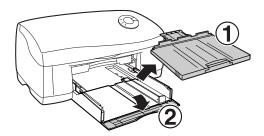
Adjust the guides ① and ② shown in the illustration to the width of the paper.
